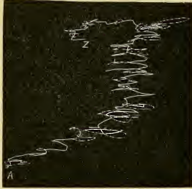
FIG. 7. — COUNTING PENDULUM OSCILLATIONS. Time of record, 80 seconds. Shows movement at first toward the pendulum, and then synchronous with its oscillations.
